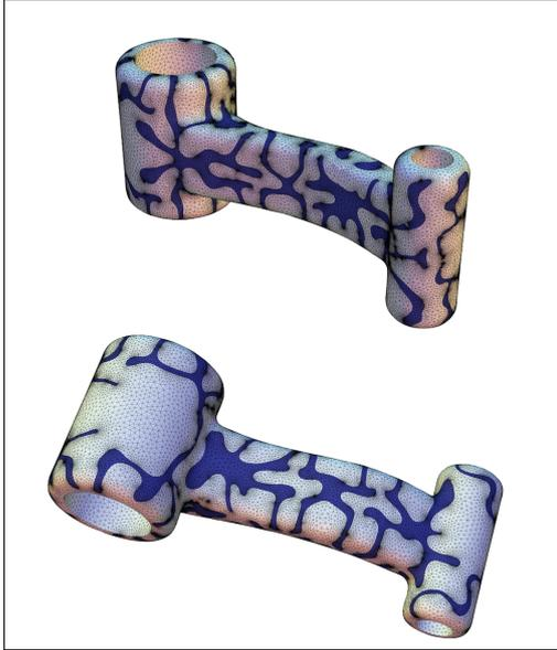
(a) Optimized design ( $n = 40$ ) in the boundary optimization process of the mechanical device considered in Section 4.2.4 with penalization parameter  $\ell = 0.01$  and mesh size  $h_{\max} = 0.08$ .
