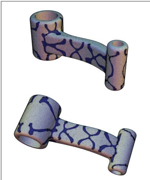
(c) Optimized design ( $n = 60$ ) in the boundary optimization process of the mechanical device considered in Section 4.2.4 with penalization parameter  $\ell = 0.01$  and mesh size  $h_{\max} = 0.05$ .
